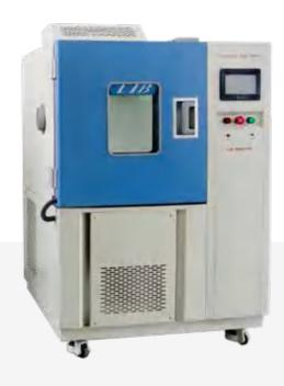
The rapid rate thermal cycle chamber is designed for testing specimens under the rapid temperature change. LIB TR models meet the ESS (Environment Stress Screen) test. The temperature ramp rate is controllable at 5 °C / 10 °C / 15 °C per minute.
